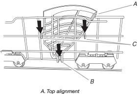
*B. Bottom slotted guide C. Knife holder hooks*
